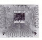
PDP-1 Module. Circa 1963 PDP-1 logic module in excellent condition. This  $5'' \times 7''$  board with its discrete transistors and resistors in shades of blues and rusts makes an interesting conversation piece, and provides a useful reminder of computer components.
